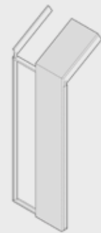
Light Metal Framing with Opaque Insulated Panel
