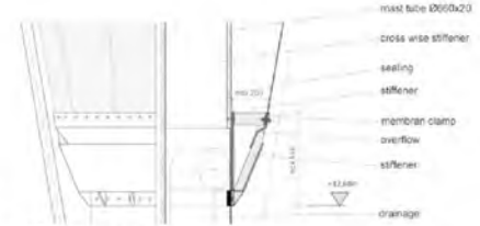
detail 2.05: drainage scale 1:10
