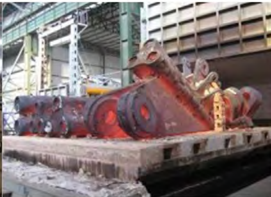
Casting Steel Joints
