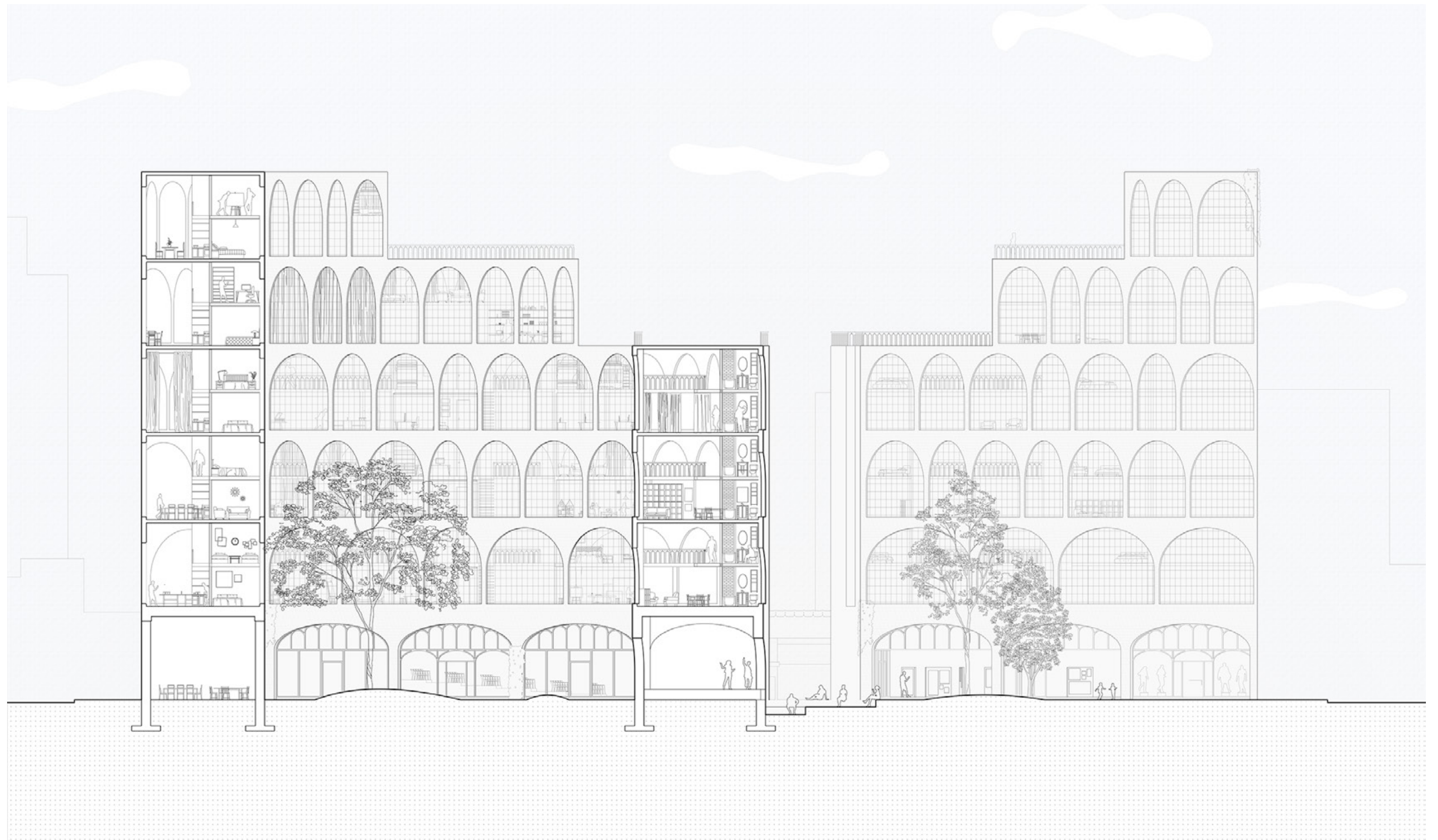
North-South Section of eastern building
