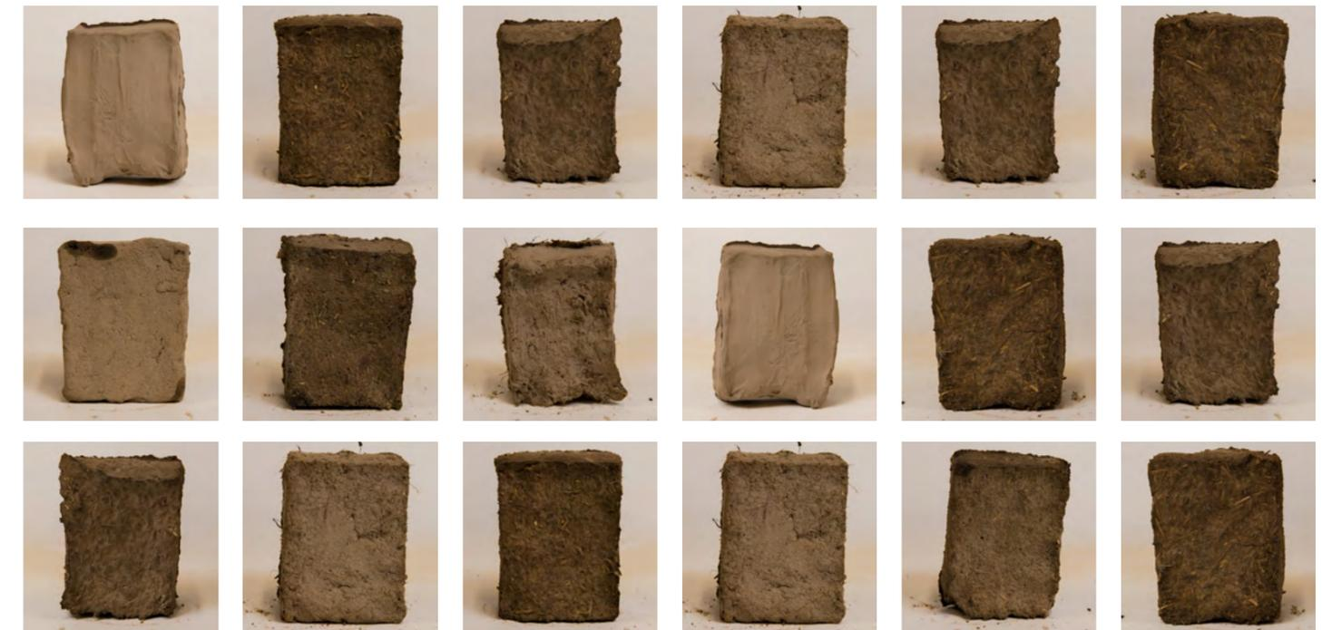
Jandug consisted of many different mixtures each with its own ratio of clay to sand to water to straw, and each with its own physical properties and role. For instance, the outer finish consisted of mostly finely sieved clay to ensure that it appears very smooth, and work well against cracking.
