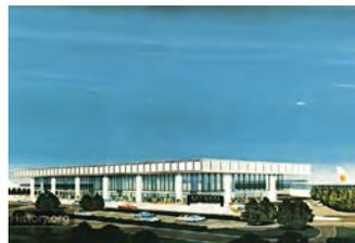
I.M. Pei markedly simple design featured a straight, flat, 600 foot aluminum-sheathed roof, supported at the edges by concrete pylons two levels high. The building was enclosed on all sides with glass for a feeling of openness.
