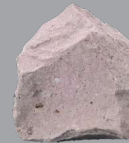
Rhyolite Igneous, volcanic rock, of felsic composition. It may have any texture from glassy to aphanitic to porphyritic.
