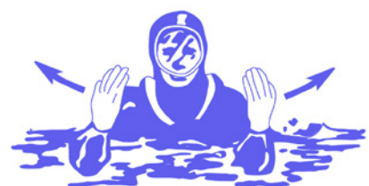
LOWER BASKET CRADLE FOR PICK-UP (CRADLING MOTION)
