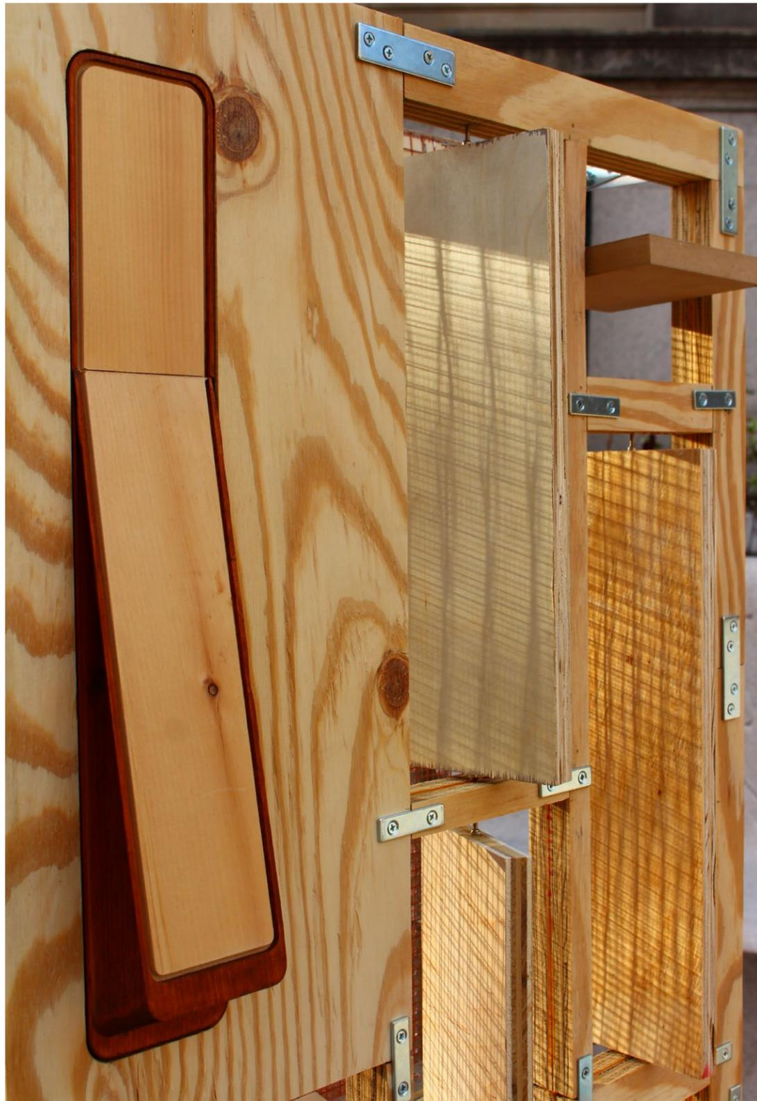
The door handle is fabricated with CNC milling, the curve on the back and the angle give the ergonomic grasp to the users.
