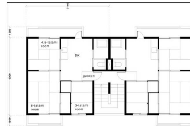
Fig1.1 Wakamiya Danchi: two 3DK units in a typical one-staircase building plan
