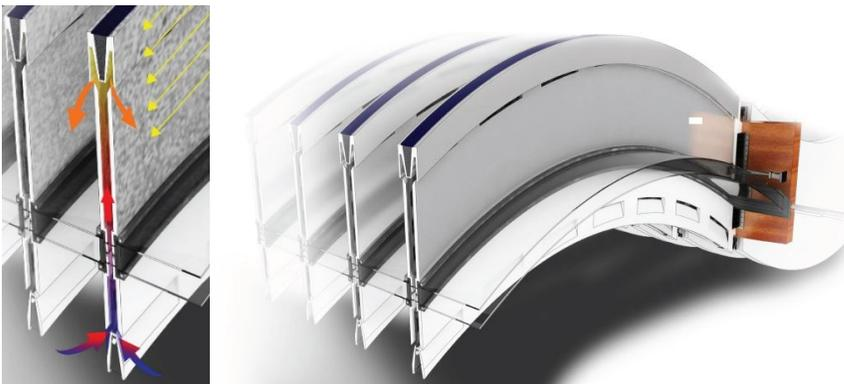
Proposal: Yan Chan, *Architecture of the Creative Space: Roof Beam as PV and Powerwall: photovoltaic strip, battery and air-exchange.* Columbia GSAPP, Mike Pilliod, Wills Sweney, Tesla, Spring 2016.
