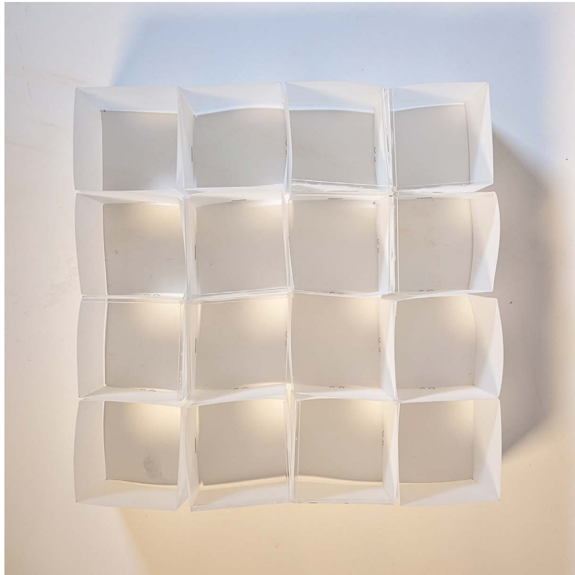
An initial material study used heat to deform a network of mylar tubes and examined how adding acrylic rods helped reduce deformation.
