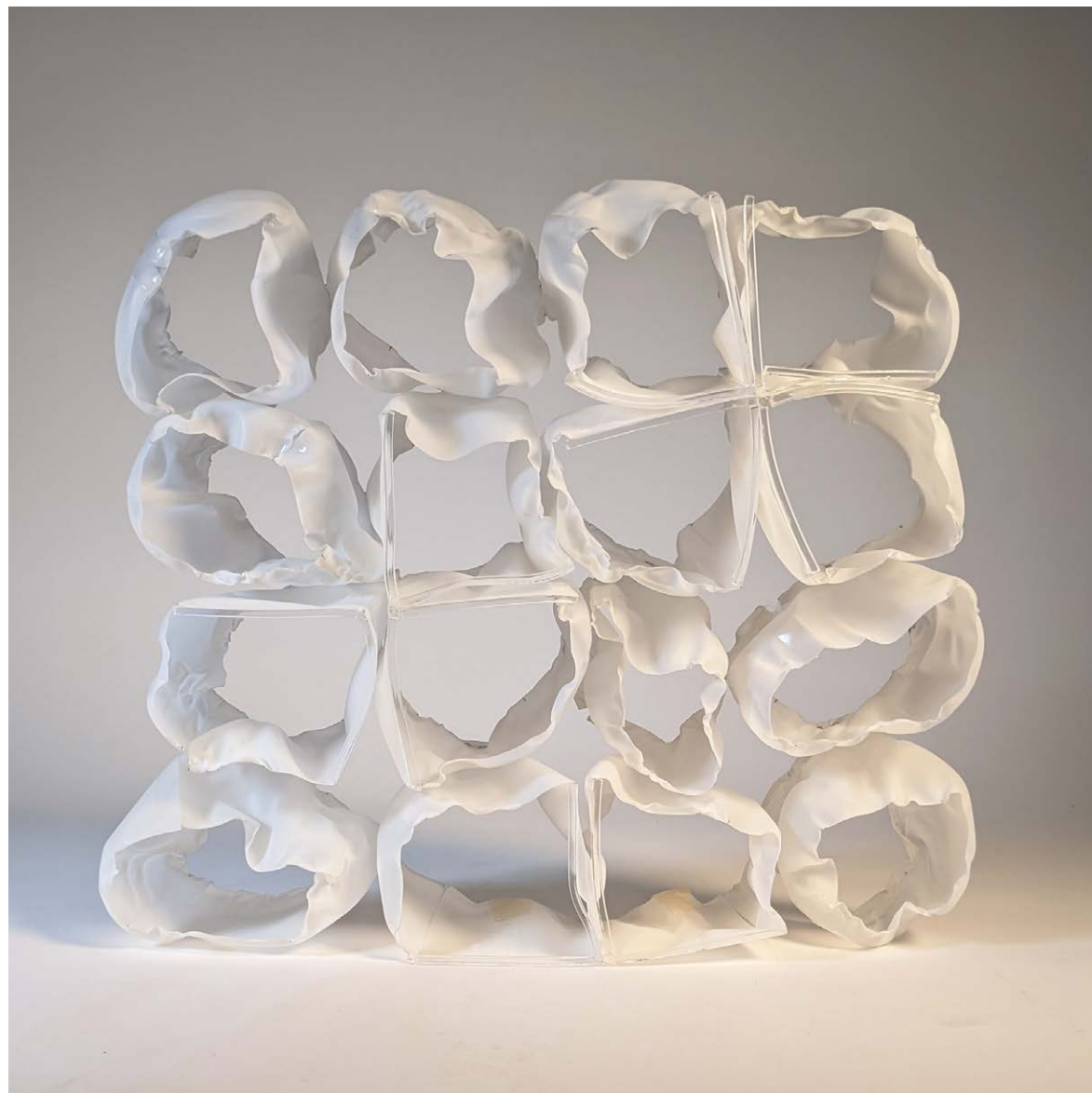
An initial material study used heat to deform a network of mylar tubes and examined how adding acrylic rods helped reduce deformation.
