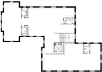
Cleared layout (ducts and washrooms retained)
