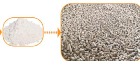
3. Cellulose powder is added to dust, and material is formed and stored as pelletized filament
