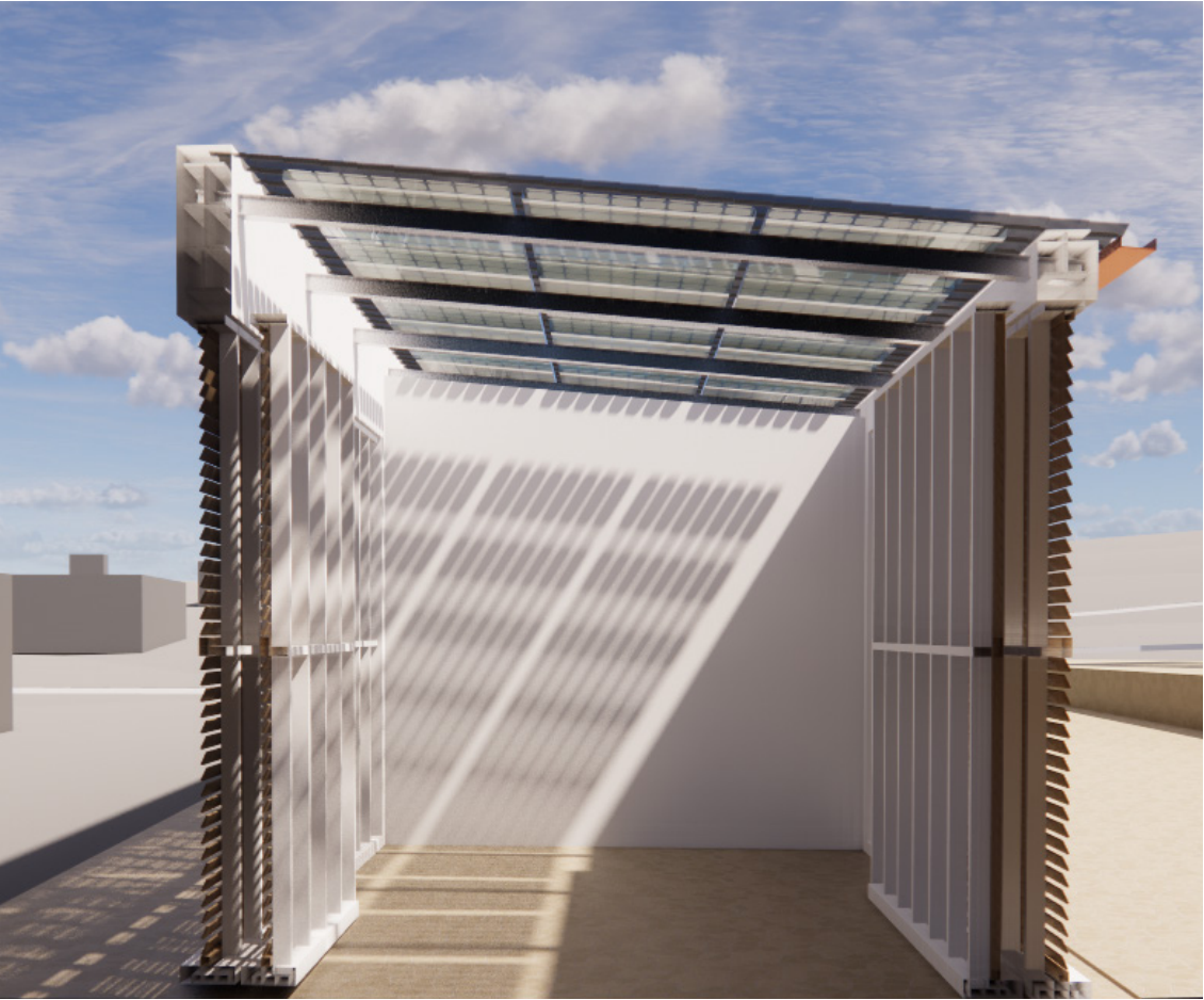
Figure 181: Steel Structure Section The section shows the interior spaces created with the steel structures and rooftop solar panels. Sliding doors and translucent panels help create a more open space where visitors can peak into indoor spaces.
