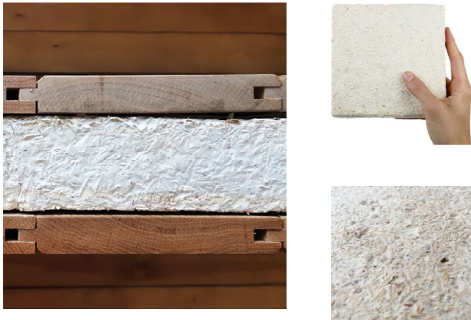
FIG. 5 Mycelium products by Ecovative used in construction (left) and for packaging (top-right); detailed view (bottom-right)
