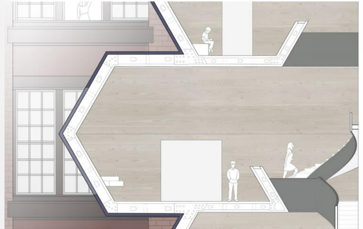
*Detail at intersection - CFS framing*
