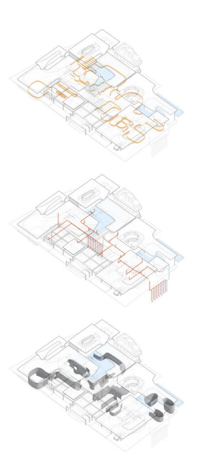
The three images are, in order, the exchange ducts, the floor heating and the damping wall. They contribute to the temperature maintainance of the whole building.
