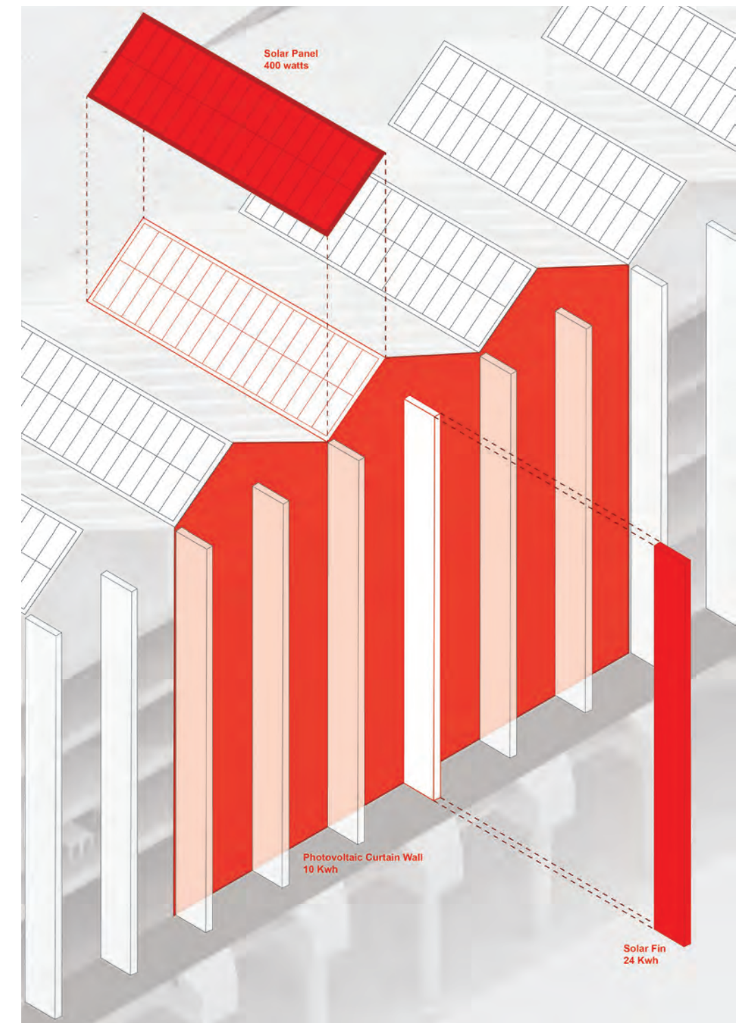
Building Material Axonometric Motorgate Parking Garage Photovoltaic Glass + Fins / Solar Panels
