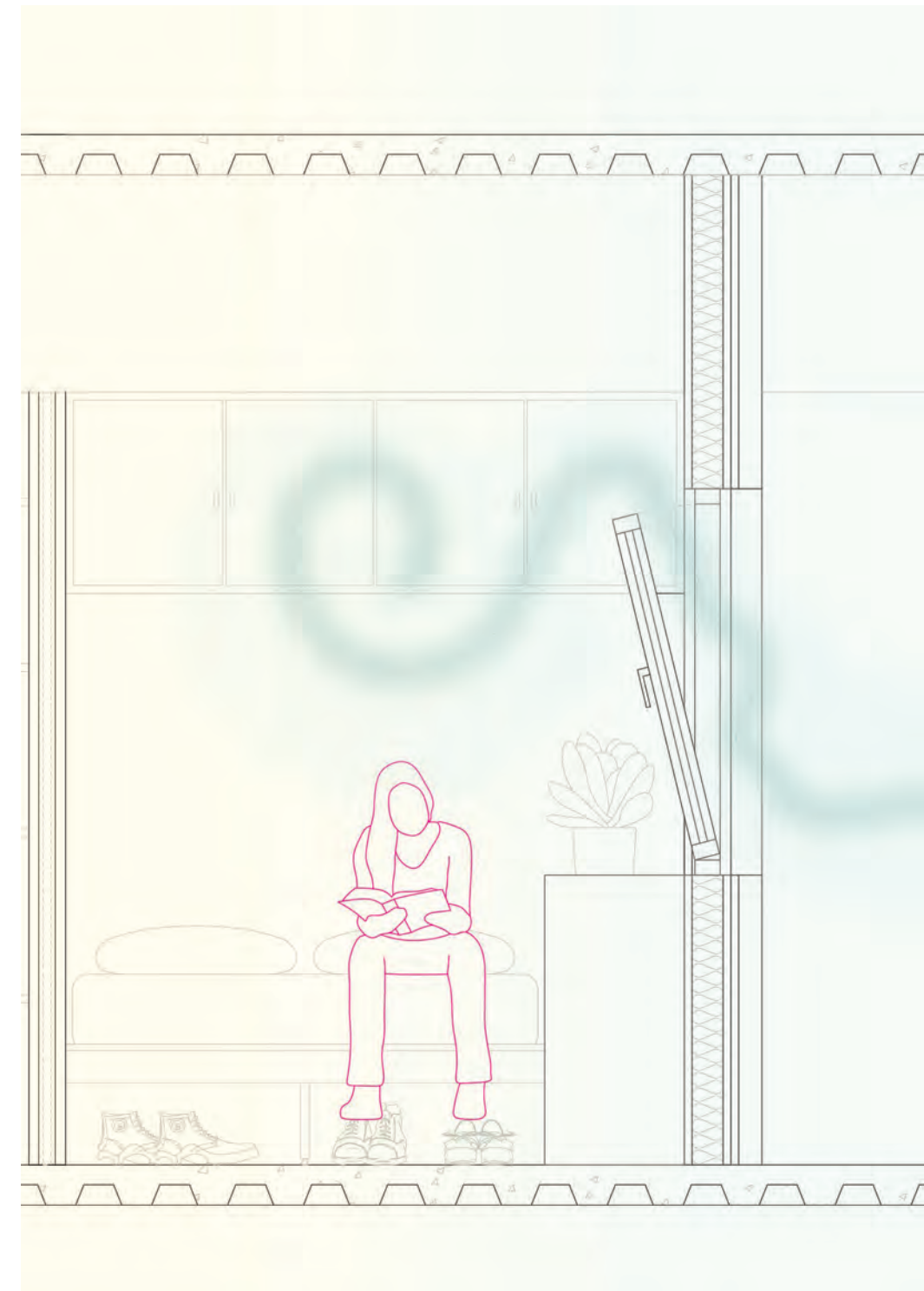
Cross Ventilation Diagram Tilt Turn Window
