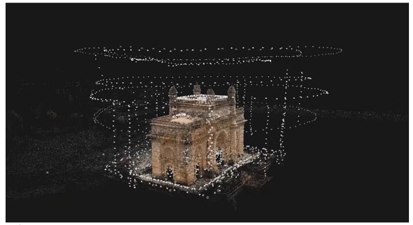
**Data Processing** LiDAR, terrestrial and aerial photogrammetry of the site is aligned with precise GPS control to create a single 3D photo-textured surface model which can then be used as a basis for producing derivatives and further analysis. **Video Credit: CyArk Foundation**
