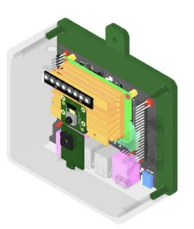
Image (bottom left): Model enclosure and harware parts laid out. Using online available STEP files to create a precision enclosure
