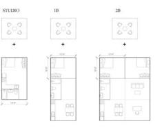
The minimal living module to accommodate daily activities is defined as 12\*10. All four types of units are made up with the basic modules of bedrooms, living room, kitchen, bathroom, and most importantly the access to an outdoor terrace .
