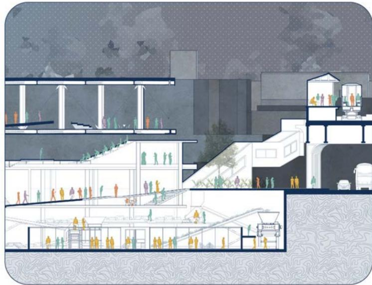
Long section with view of underground recycling center, sunken level corridor, outdoor amphitheater and truss bridge.
