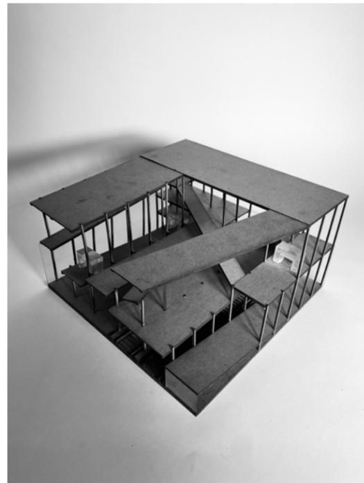
The design strategy consists of long spanning ramps, supported by trusses, that connect different programs to each other, the different levels of the building and the surrounding context. All these ramps sectionally overlap providing a sense of transparency and visibility into all the different spaces of the building. This reinforces the idea of exposing what is usually hidden.
