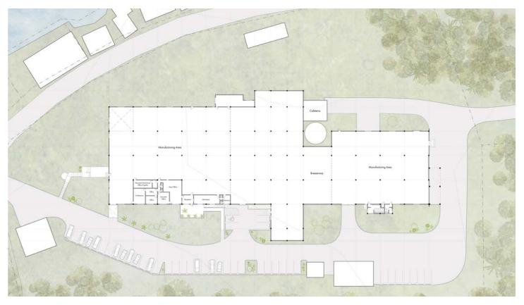
Existing Plan. The building structure is mainly composed of a column and truss steel frame with spans of 30' by 30'. It used to be the first Baxter International Company brought to Culebra in 1972. The company manufactured iv serums. It later became RD Medical after it was sold in 1996. The building is currently in disuse and owned by the government.
