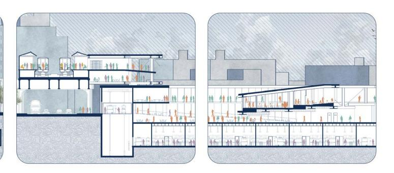
Long section with view of underground recycling center, sunken level corridor, outdoor amphitheater and truss bridge.
