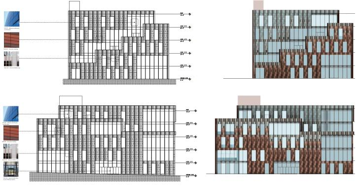
The facade system consists of a unitized curtain wall system with pre-fabricated panels made up of terracotta tiles of various colors.
