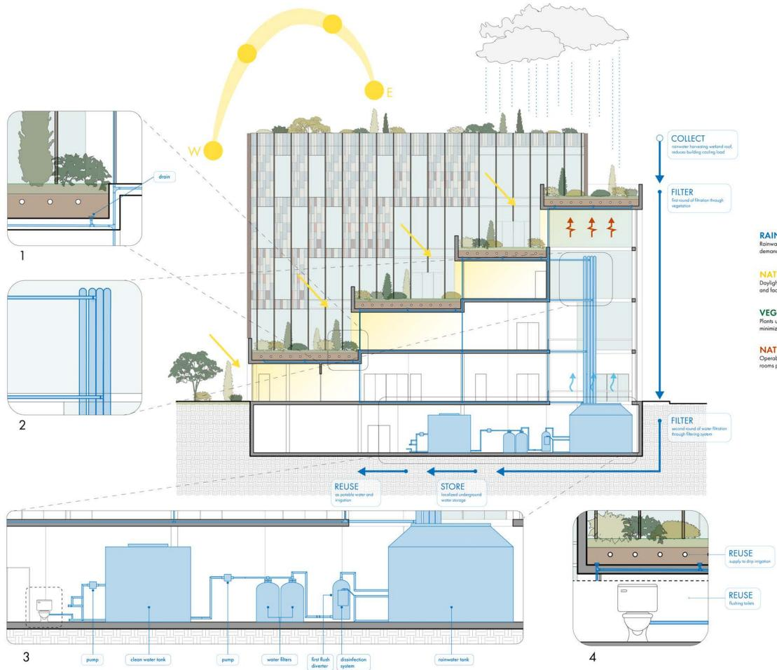
RAINWATER MANAGEMENT Rainwater management to offset potable water demand and minimize storm water runoff.
