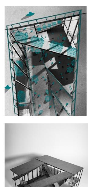
The design strategy consists of long spanning ramps, supported by trusses, that connect different programs to each other, the different levels of the building and the surrounding context. All these ramps sectionally overlap providing a sense of transparency and visibility into all the different spaces of the building. This reinforces the idea of exposing what is usually hidden.
