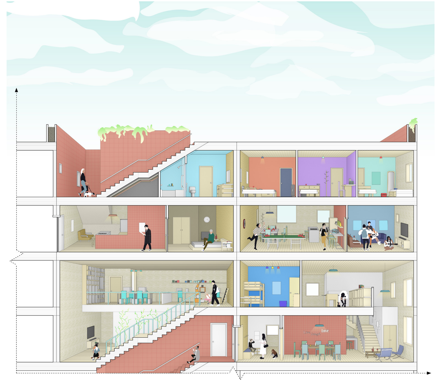
The cork-clad CLT shear walls of the 2-storey modules create complete acoustic segregation between units, allowing for a great diversity of work/live/study living scenerios next to one another.
