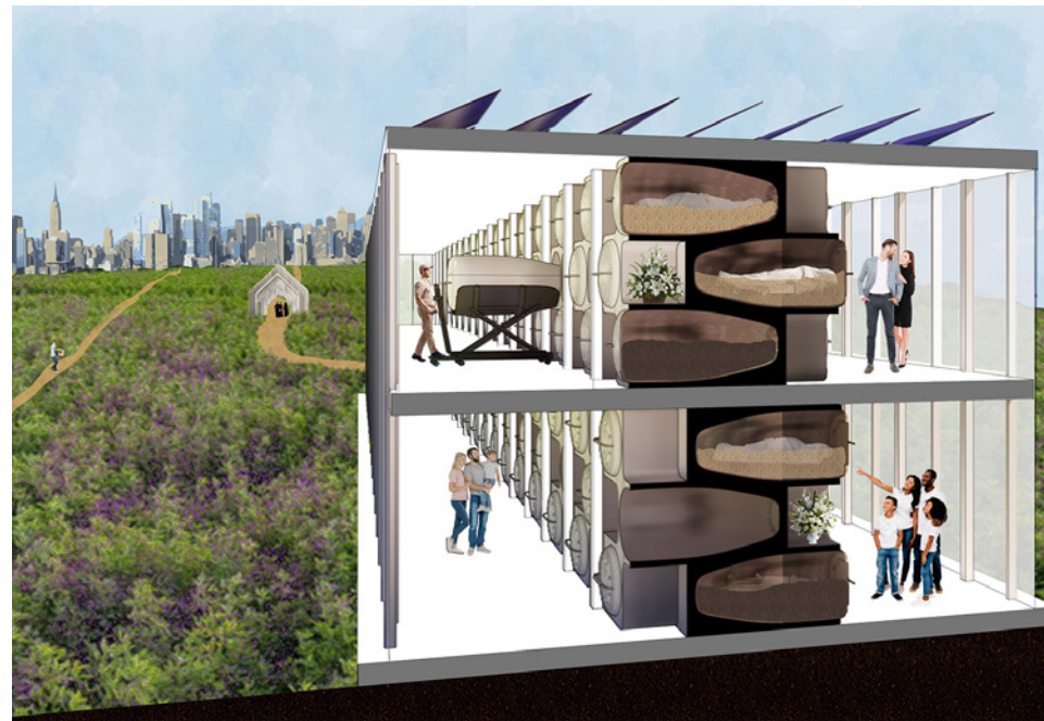
Existing cells are transformed for the terramation vessels and preserve structure, such as columns and slabs, and remove the facade.
