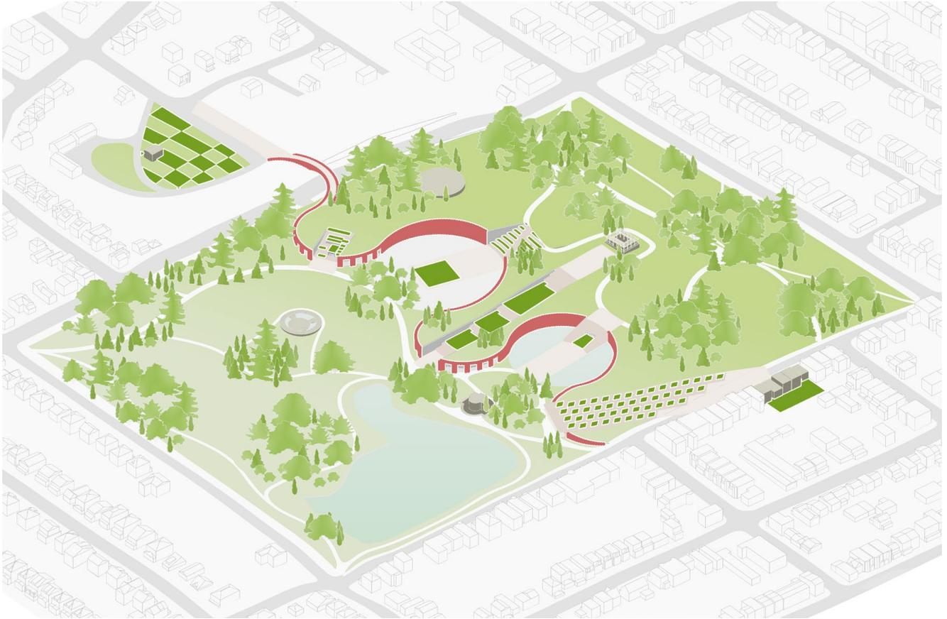
The cut-and-fill operations stitch the two side of the park, cutting out new open air playgrounds as well as building up single floor indoor spaces. The height of the wall changes with the existing topography, becoming as tall as 2-floor high amphitheatre seating and as low as below grade to allow seamless trespass.
