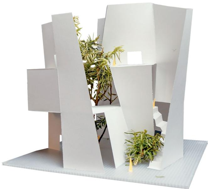
The architectural operation of folding increases exposure, creating in and out spaces interacting with surroundings in different ways: terraces of different heights extending the inner rooms to the outside, while the central atrium invites in natural light and street life.
