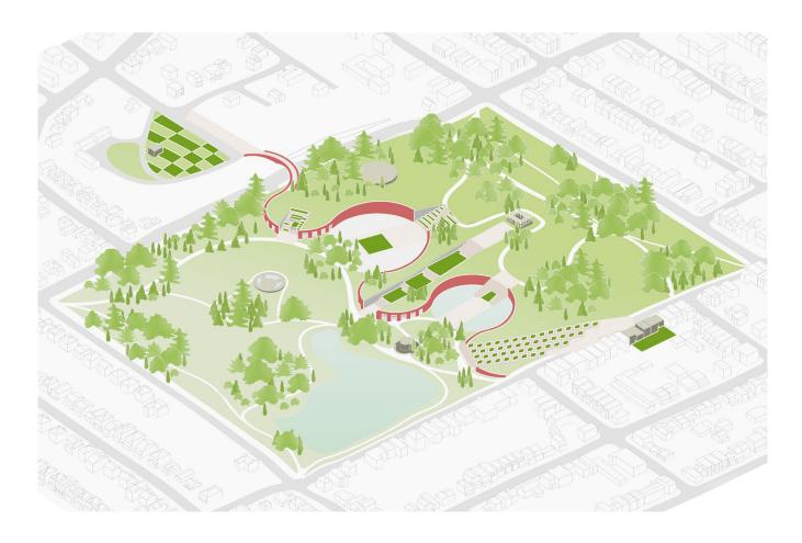
The cut-and-fill operations stitch the two side of the park, cutting out new open air playgrounds as well as building up single floor indoor spaces. The height of the wall changes with the existing topography, becoming as tall as 2-floor high amphitheatre seating and as low as below grade to allow seamless trespass.
