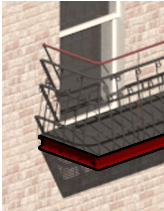
2A STRUCTURALLY REINFORCE EXISTING FIRE ESCAPE.
