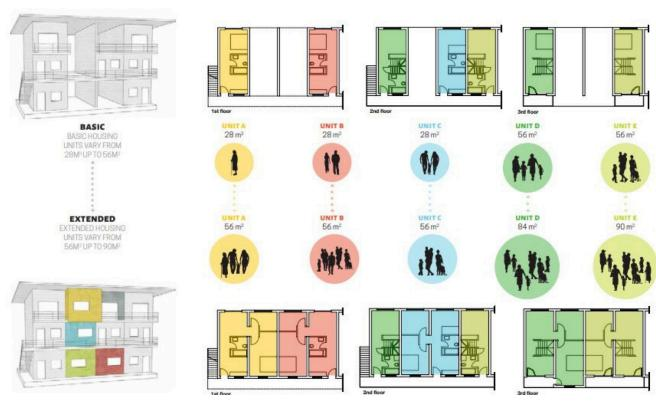
Figure 6 Drawings of Incremental housing types to be constructured
