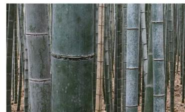
Using bamboo as building material has the strength that it is fast growing plants on the plant. Bamboo's strength-to-weight ratio is similar to timber, and its strength is generally similar to a strong soft-wood or hardwood timber.
