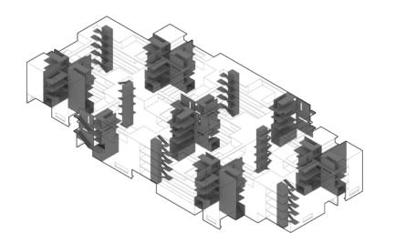
Two types of circulations are designed. Circulation 1 has relatively complicated circulations and platforms, and it is intened to be a social space for people to interact on the move. Circulation 2 fulfills the ADA requirement and efficiency.
