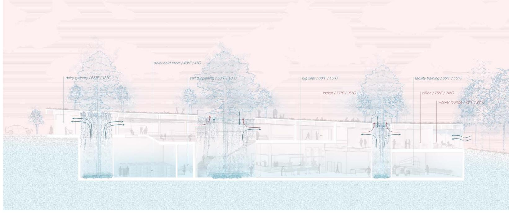
Subsoil temperature becomes stable at 20ft to 30ft below ground, which is called "Mean Earth Temperature." In upstate New York, the mean earth temperature is around 47 °F. Different programs require different temperatures. The plant takes advantage of the forest and topography by building underground for the natural cooler subsoil temperature.
