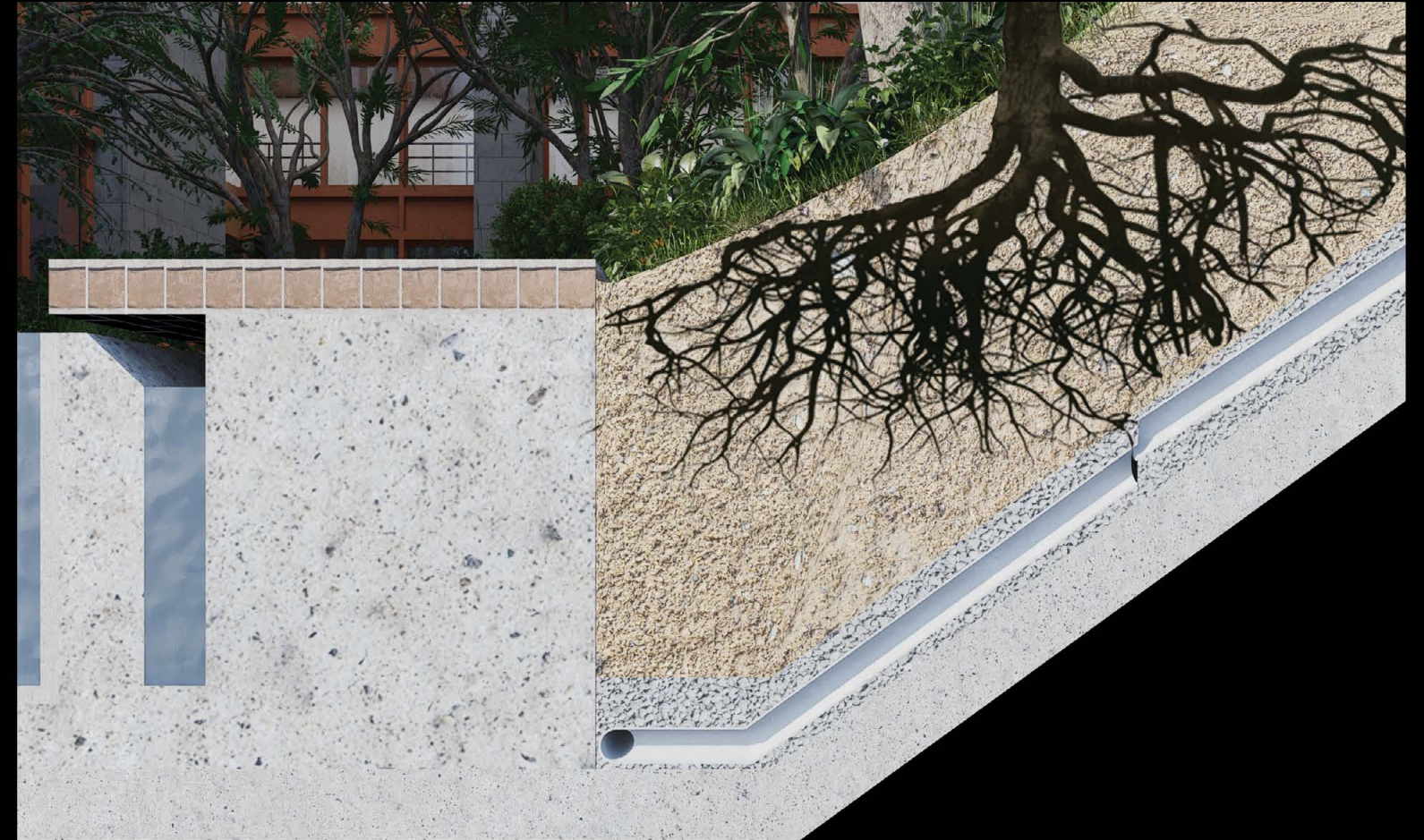
2.3. The invasion of the trees: They grow horizontally between the gaps of the bricks and they grow downwards to compress the earth and eventually break the drainage pipes.
