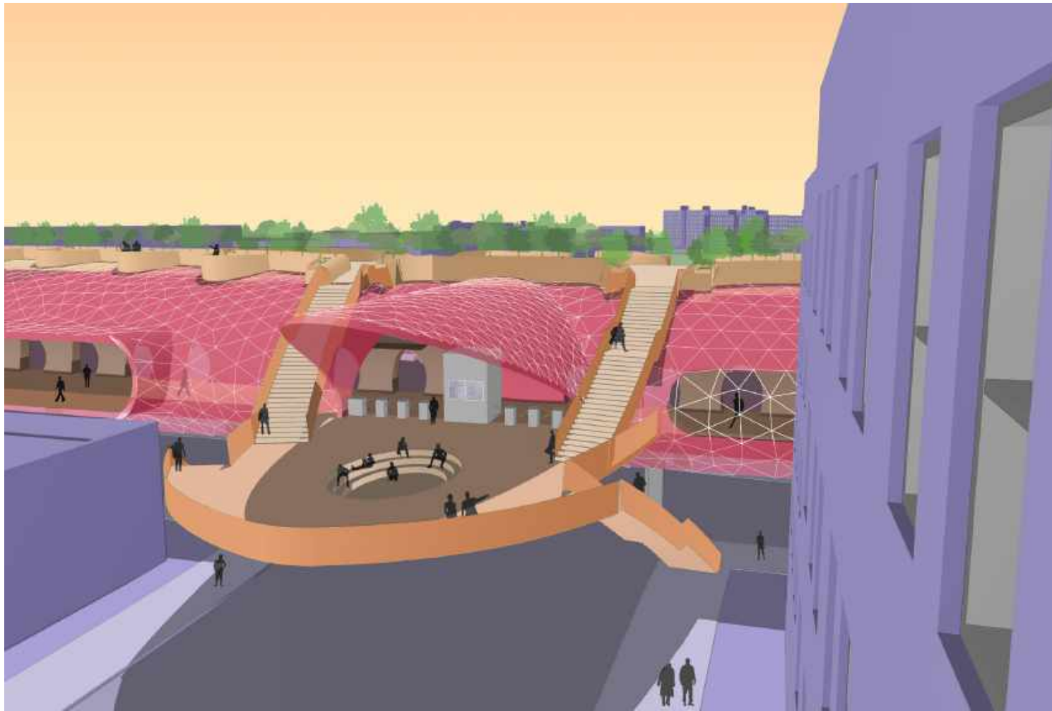
DIN-sign utilizes a geodesic structural frame to lighten the overall mass of the subway's new sound enclosure.
