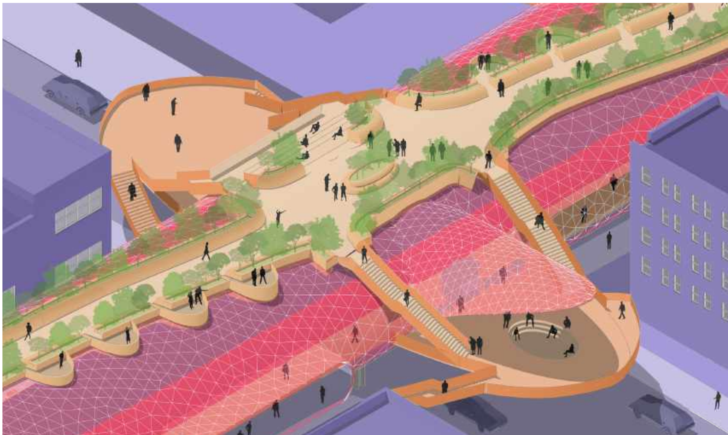
It is wrapped in a transparent canvas fabric that allows light to penetrate the interior of the enclosure during the day.
