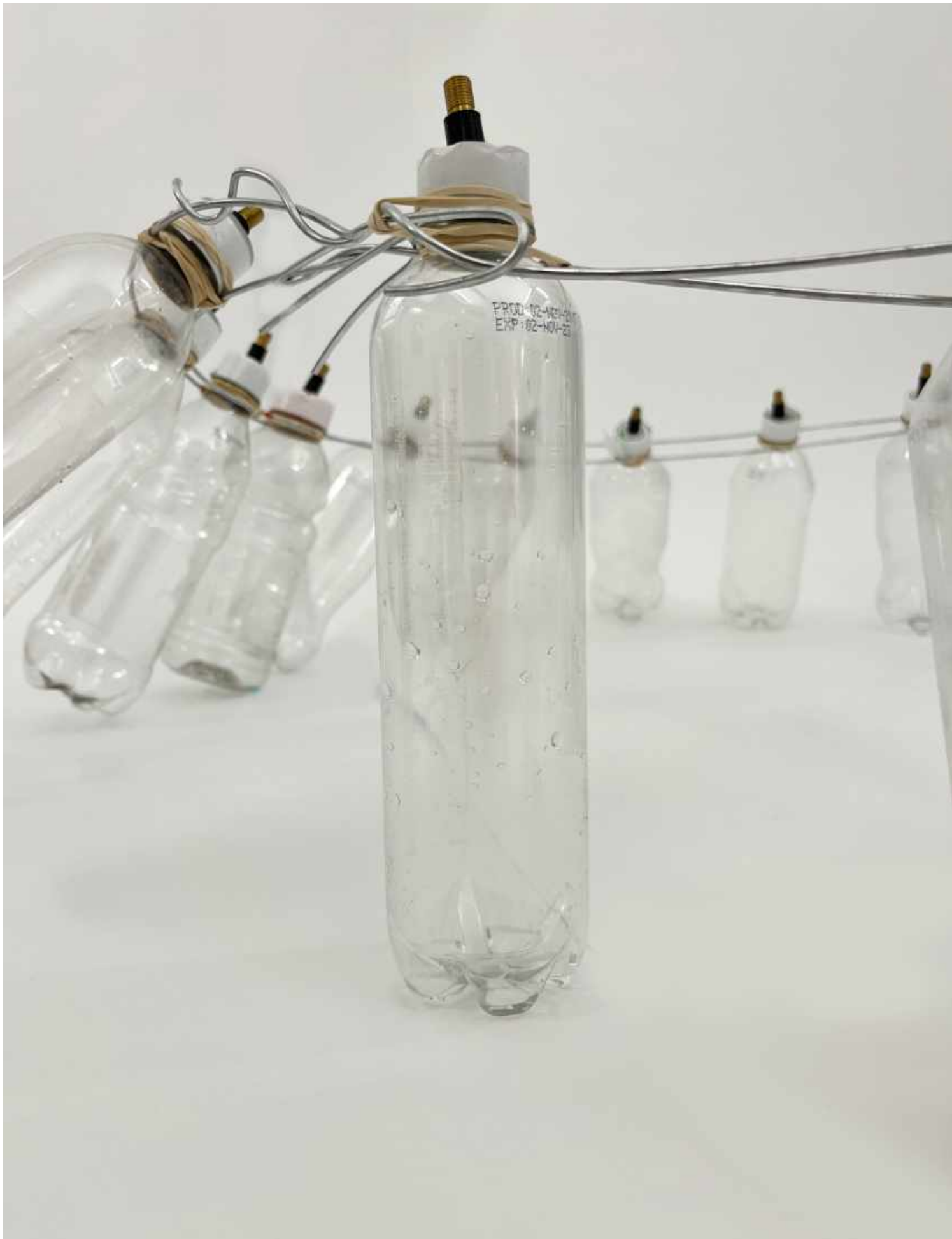
106 The bicycle valve applied to the top of the bottle allows pressure to be adjusted.
