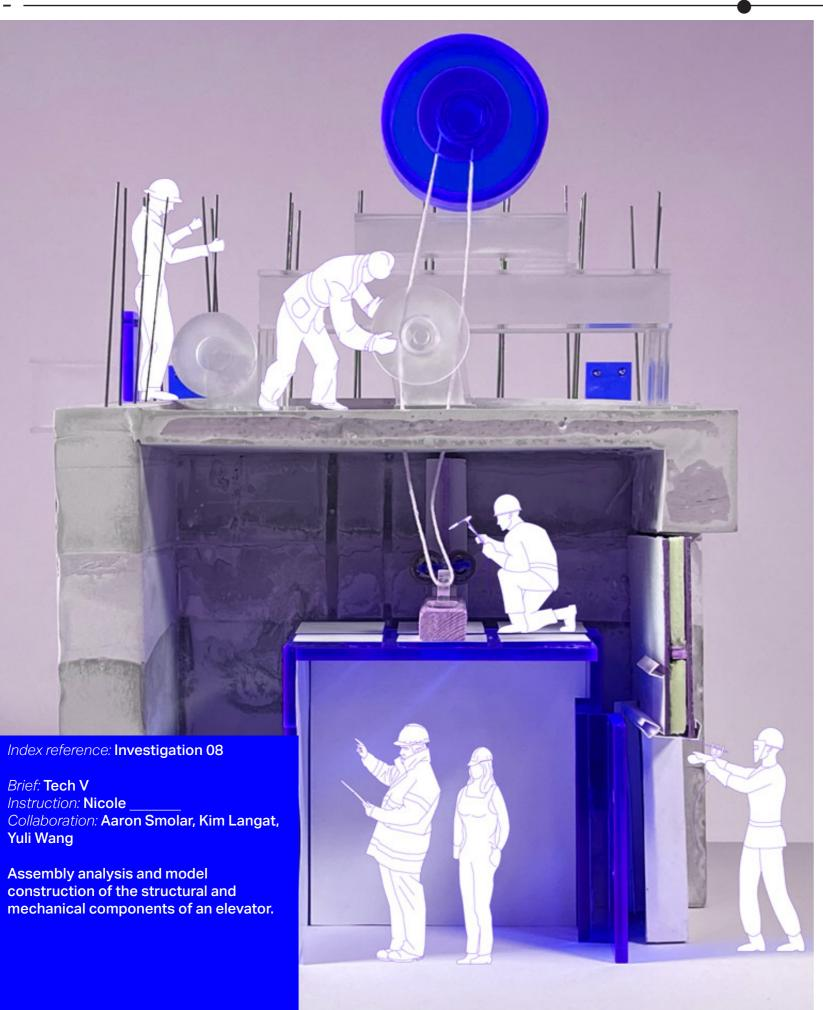
elevator cab detail with counterweight, guide rail and elevator rollers AT V GROUP C5 Aaron Smoler Kim Langat Maclane Regan Yuli Wang
