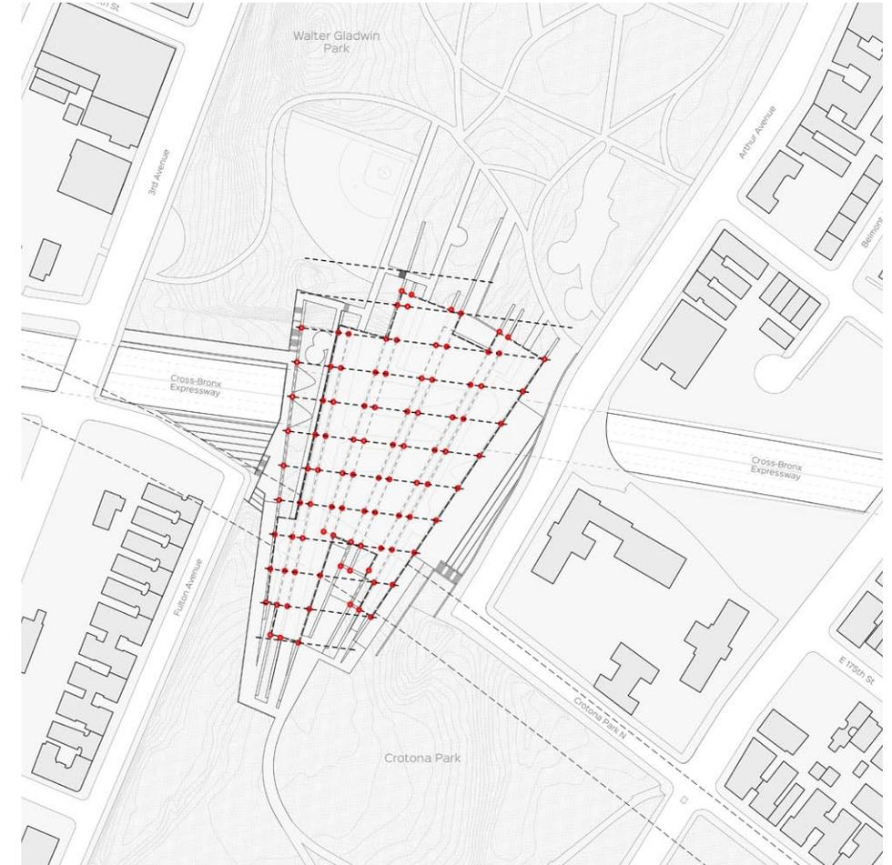
The basic configuration of the new hall takes cues from the site context. Its radial layout is defined by two curves, one perpendicular to the CBE, and the other parallel with Arthur Ave. The strips are laid out in an AB pattern—with the overlaps in the A larger strips resulting in smaller B strips.
