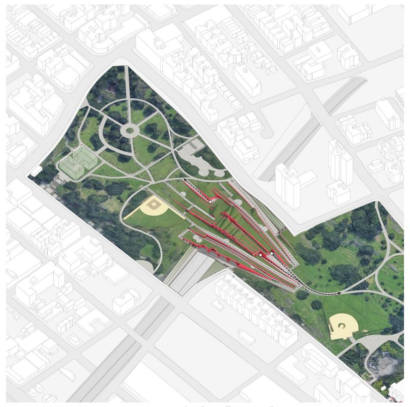
The strips have varying roof forms. Some slope down into the terrain of each park on either side of the CBE—providing walking paths via their green roofs above and spatially reconnecting the two parks. Other strips peel upwards and provide access directly from the ground level of the market hall.
