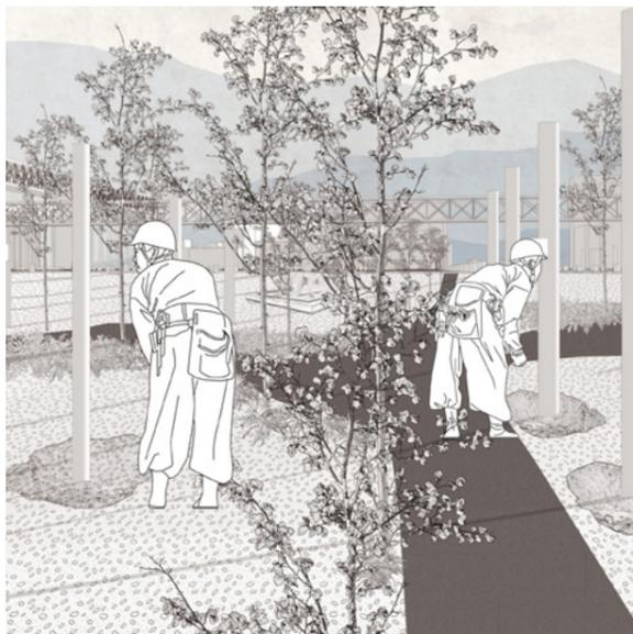
Phase 1: We regularly implant air sparging equipment in the venue. They are mainly in the form of pipes that go deep into the ground, so in order to insert them into the site, it may be necessary to remove some of the existing paving and green space in the park.
