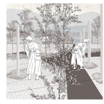
Phase 1: We regularly implant air sparding equipment in the venue. They are mainly in the form of pipes that go deep into the ground, so in order to insert them into the site, it may be necessary to remove some of the existing paving and green space in the park.
