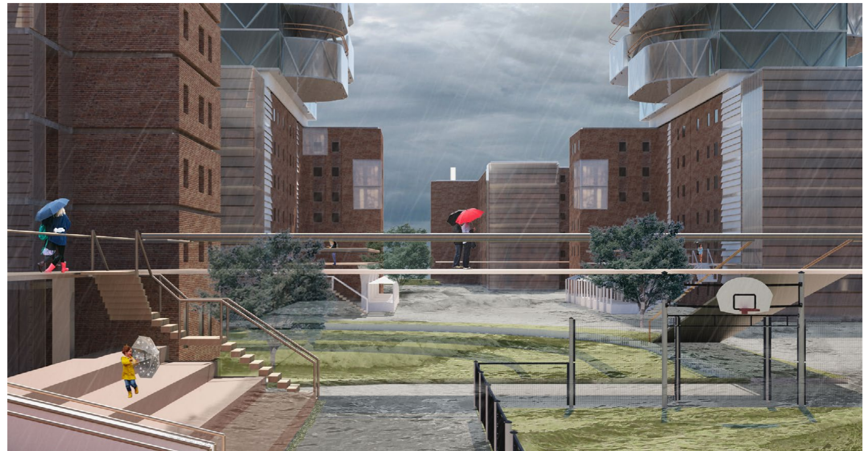
When it is raining, the ground floor will serve as barrier to resist the rising river and residents will use hallways in the air to walk.
