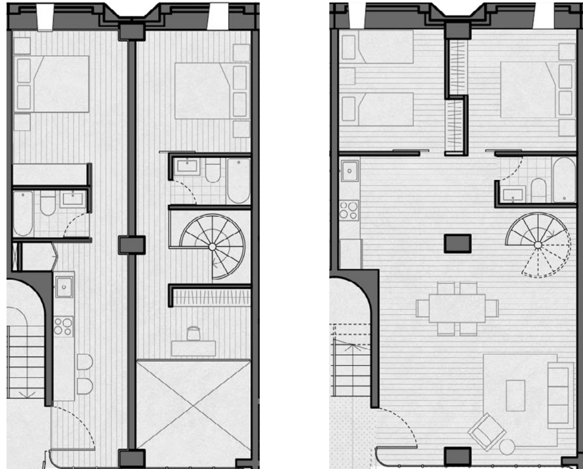
Duplex and double-sided units. Common spaces facing alcove and bedrooms facing original facade with smaller openings. Produced by authors.
