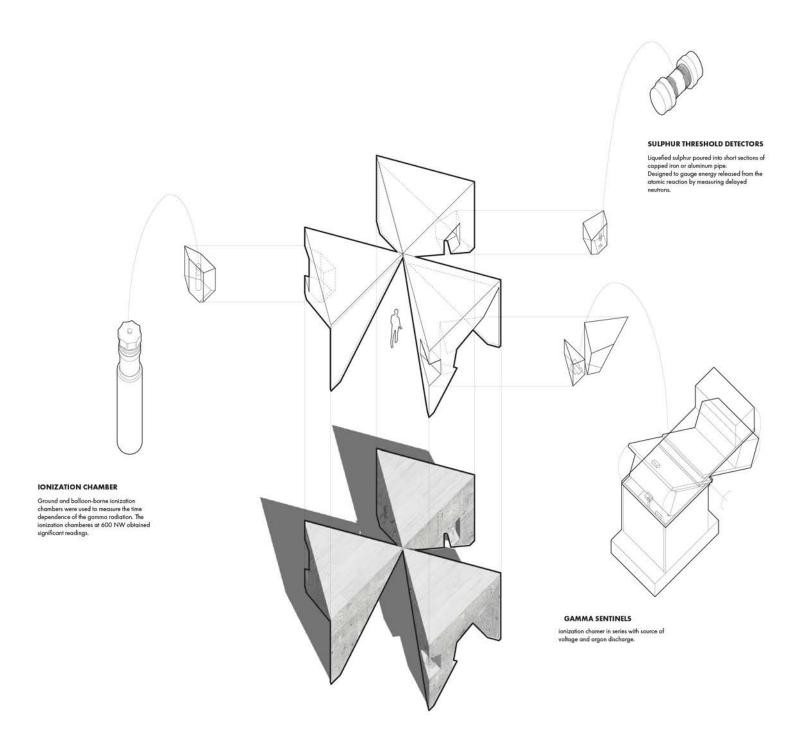
The energy released from the atomic reaction would be gauged by recording delayed gamma rays in ground and airborne ionization chambers, with information transmitted to the three 10,000-yd bunkers. Eight sulphur threshold detectors and a number of gold-foil detectors would also measure delayed neutrons.
