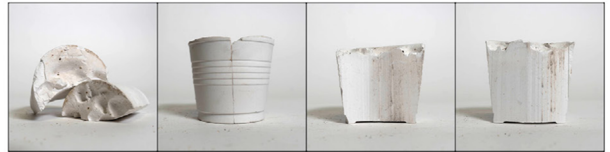
(01) TEMPORARY AGGREGATE: ICE
