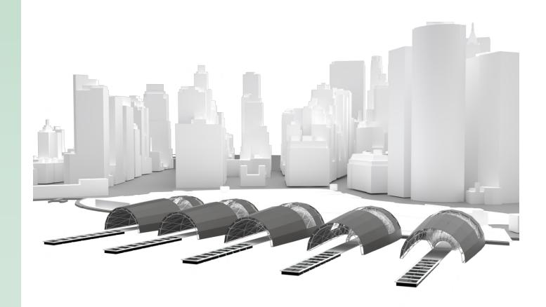
350 W PV PANEL : ABOUT 2858 PANLES TO GET 1 MW OVER 5 PIERS WITH EACH PIER HOLDING UPTO 1000 PANELS
