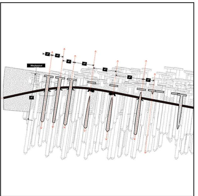
Detail of Nails and Joints that create a Fabirc
