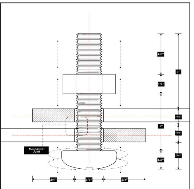
Section of screws and nuts
