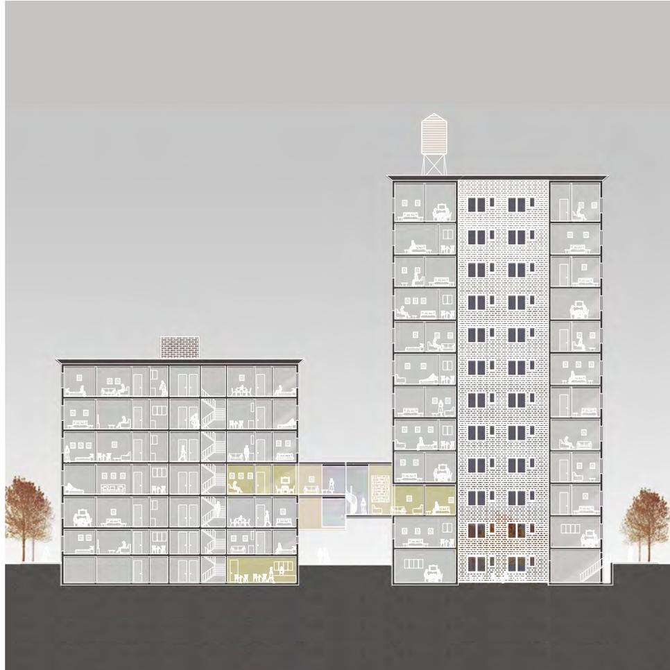
Cross section of through-block housing unit connecting existing apartment buildings.
