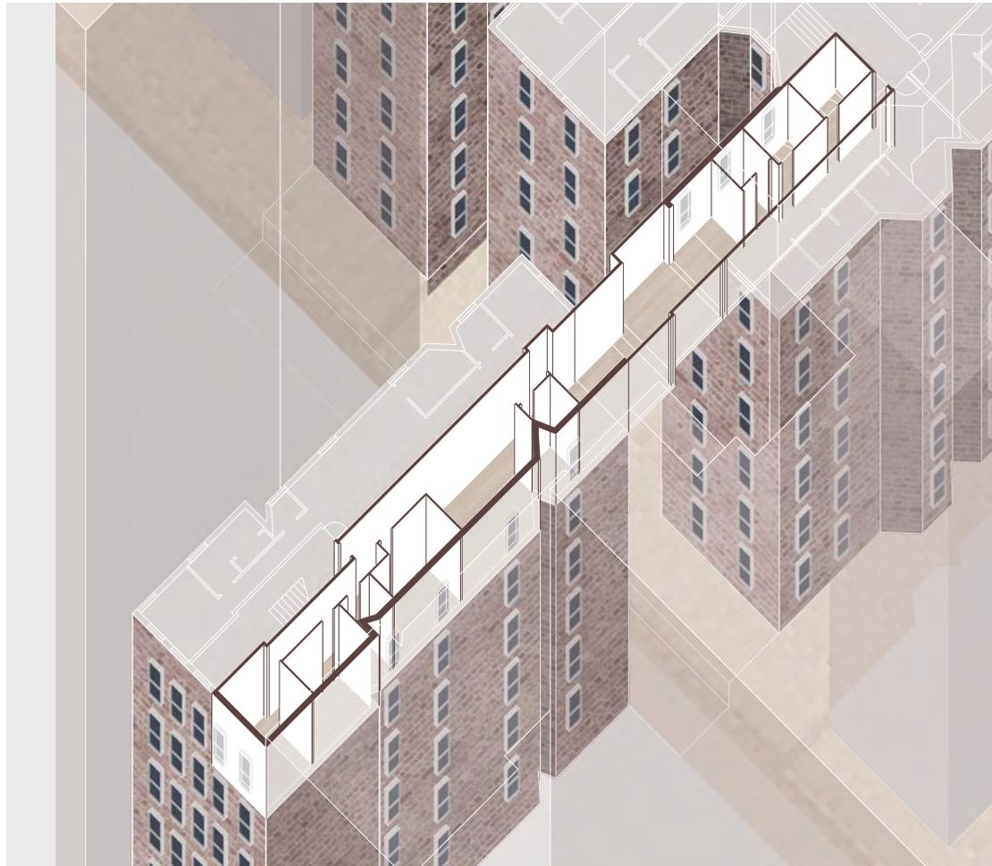
Through-block unit connecting two existing units in separate buildings on opposite sides of the block.
