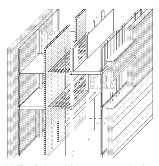
Section oblique cut through one wing of H-Block showing how the typical exterior walls have been delaminated to create occupiable spaces between the various layers of materials & systems.
