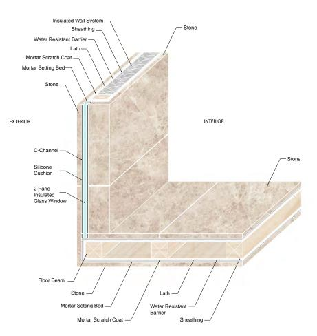
Detail drawing of corner condition of bridge portion of through-block housing units.
