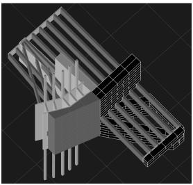
^1:1 construction model of existing building connection to proposed facade system
