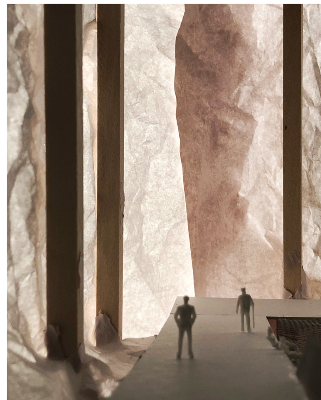
In Creating architectural model, craft paper as ground, wood stick as the building's existing columns, clay as its foundation, paper board as solid ramps were used to create industrial and substructural atmosphere.
