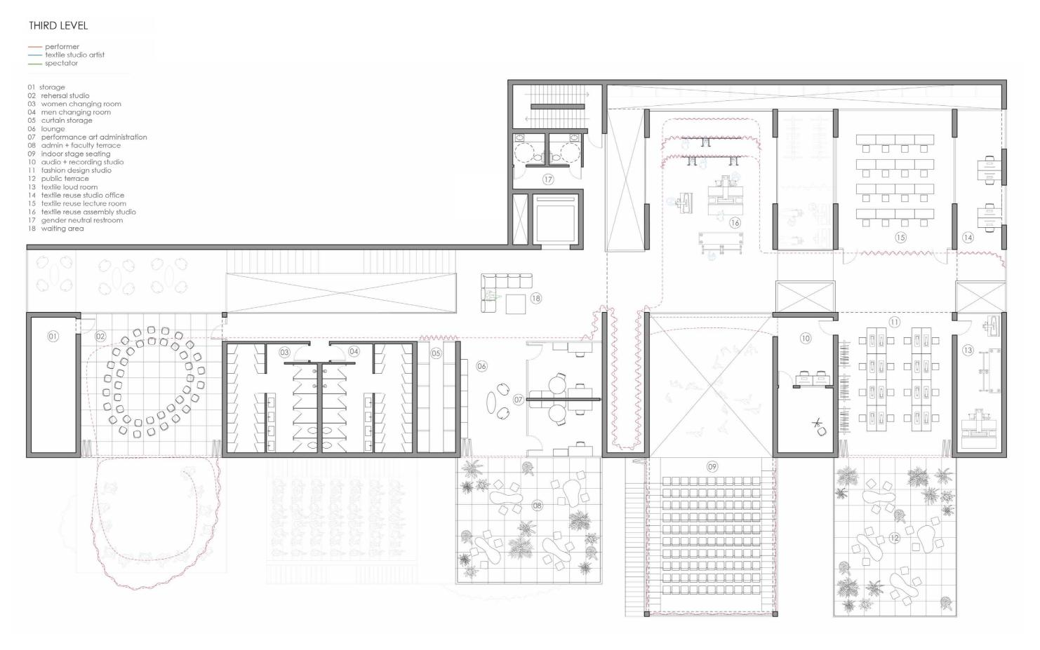
The flow of the curtain around the building aims to blur the boundary between inside and outside to create transformable performance spaces. To create a continuous transition between spaces, curtain tracks are installed to fully blend in flush with the ceiling.
