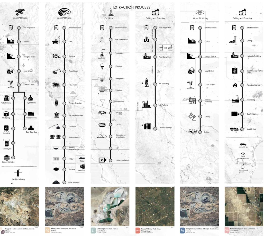
For lithium extraction, saline water is evaporated and filtered for salt, and further refined for extraction of lithium. The evaporation takes place in regions that are arid and with low precipitation rate. The entire process of extraction to finished products to consumers requires a collaborative effort from a huge network of companies, factories and transportation.
