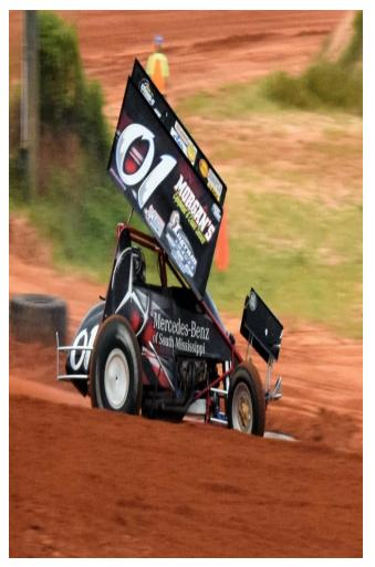
The car is a 2009 J&J Chassis and races within the ASCS & USCS series sanctions. It has a 362 Chevy 680 hp fuel injection engine, and was designed by Mc Murtry Engine
